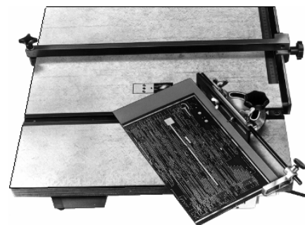
To use shear by hand, remove shear from the table unit.
