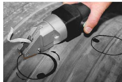
starting hole 12-14 mm Ø accurate cutting along a marked line
